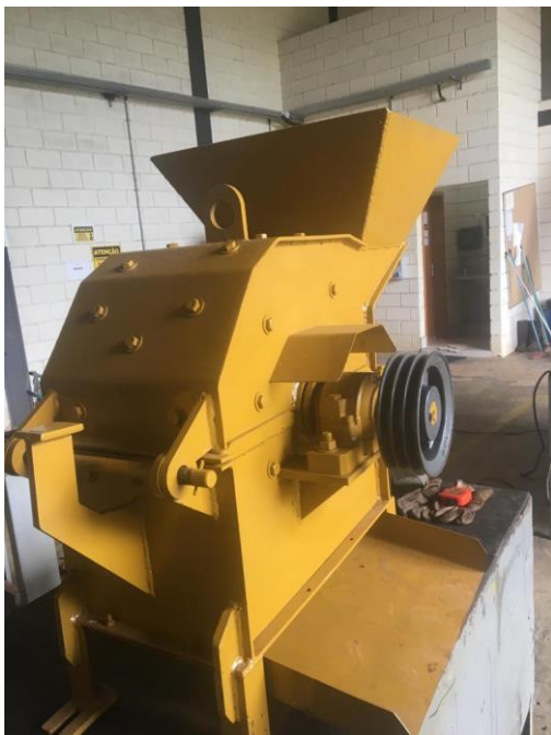
Figure 1. New Hammer Mill being installed with engine
