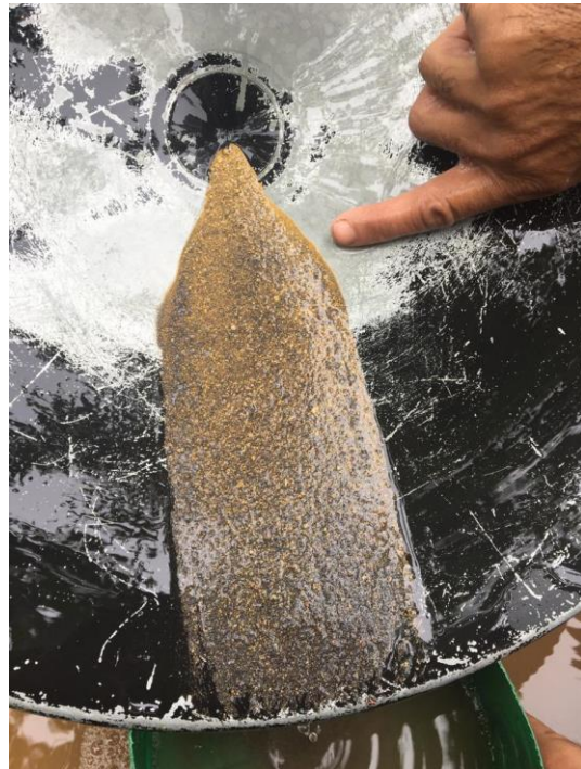
Figure 6. Hammer Mill 2 gold from panning
