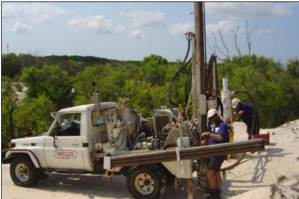
Figure 8: Drilling for sand using a typical 4WD mounted aircore rig
