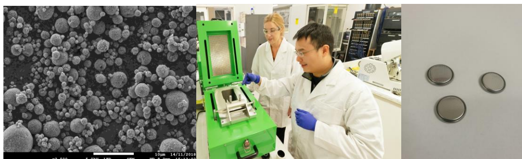
Figure 1 – VSPC LFP SEM image Figure 2 – Cell-making in the VSPC lab Figure 3 – coin cells
