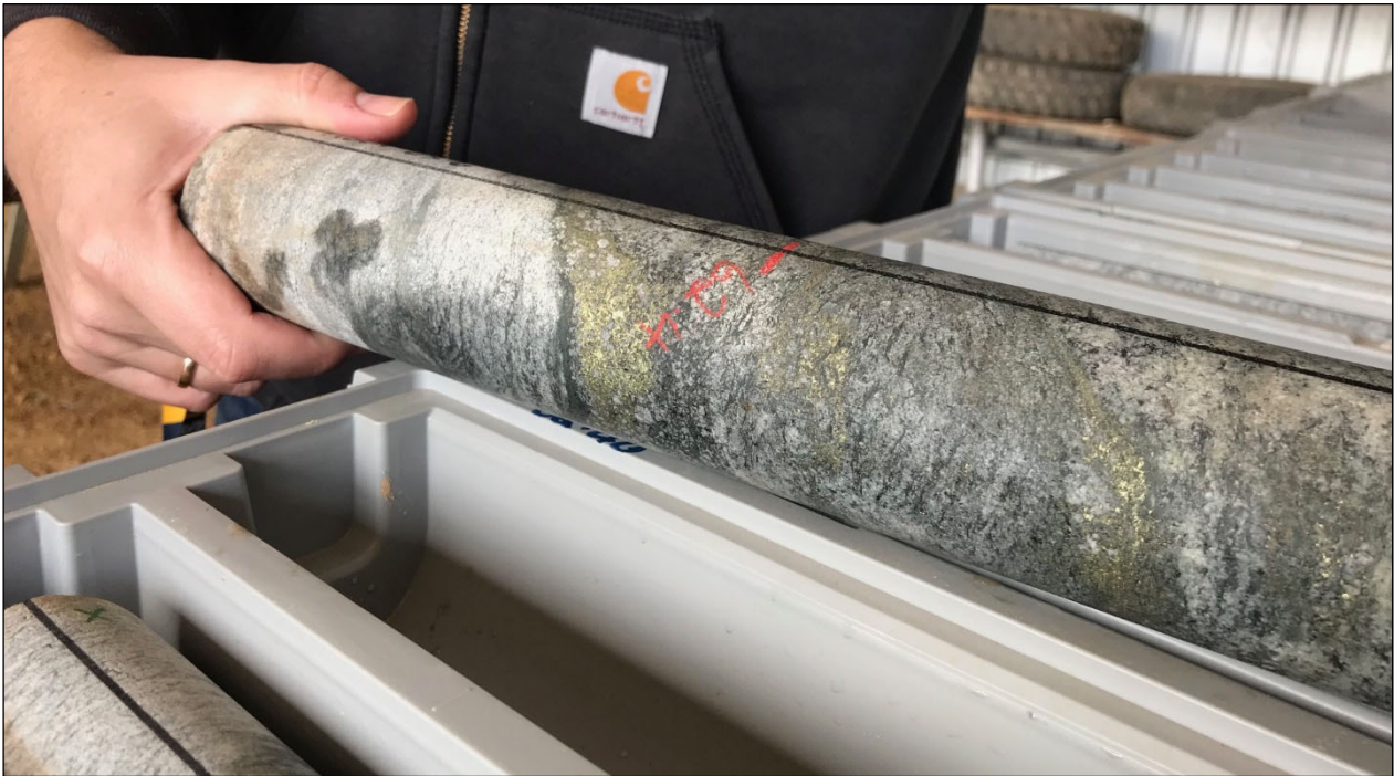
Figure 2: Chalcopyrite mineralisation from higher grade domain within Bindi West resource, intersected in diamond drill core from hole 18CAD001 at 62m depth.
