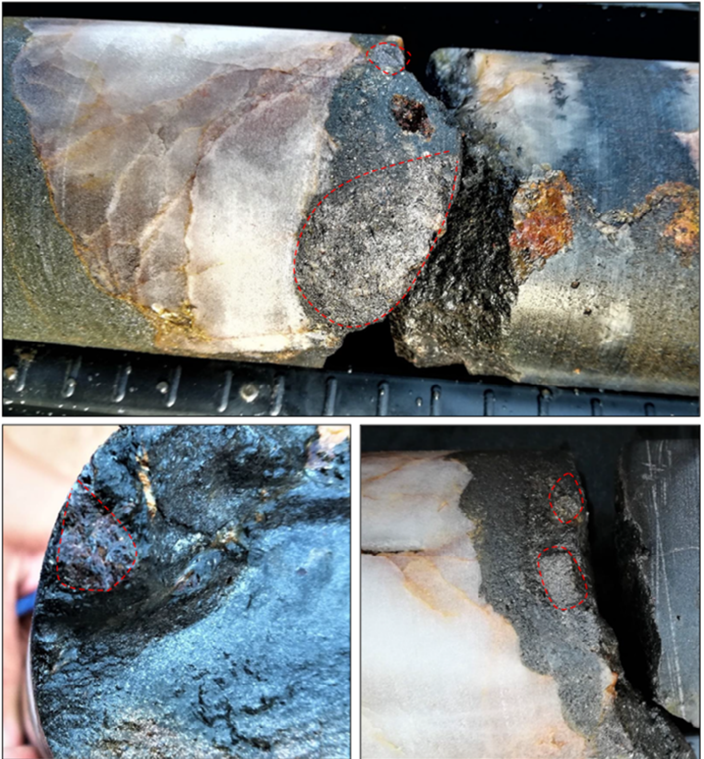
Figure 1 Cassiterite crystals seen in the muscovite-tourmaline alteration selvage to a quartz vein in KKDD003.
