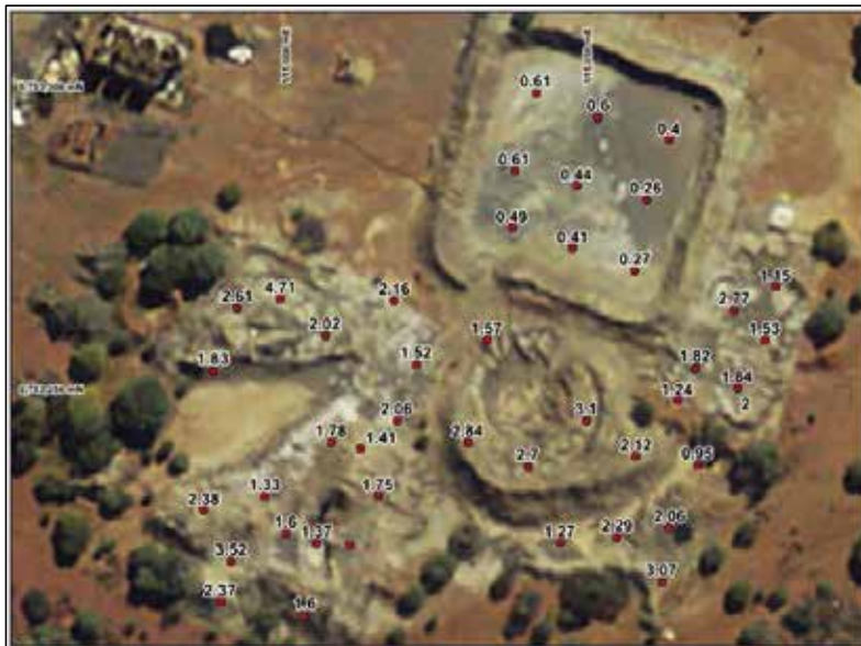
Figure 4-17: Locations of auger holes in the historic tailings area at Reid's Ridge, with gold grades from Aphex Minerals
