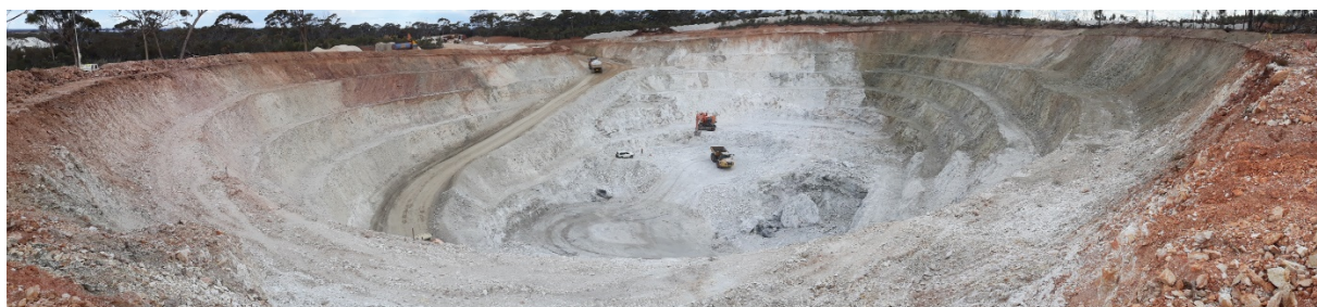
Photograph 1 - 25 th November 2018: Panorama of the Stage 1 Sinclair Mine looking South. Mining equipment includes a 75t excavator and 4 x 40 tonne articulated dump-trucks (moxies), plus drill and blast equipment.
