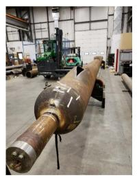
• <u>Cooled Burst Test after Fatigue</u>: This test requires fatiguing the specimen through 3 times the design life (6,000 cycles) and then bursting the pipe after it has been cooled to simulate the temperatures that would result from the Joule-Thompson cooling effect of gas escaping through a crack. This test has commenced and will take about 14 days to complete.
