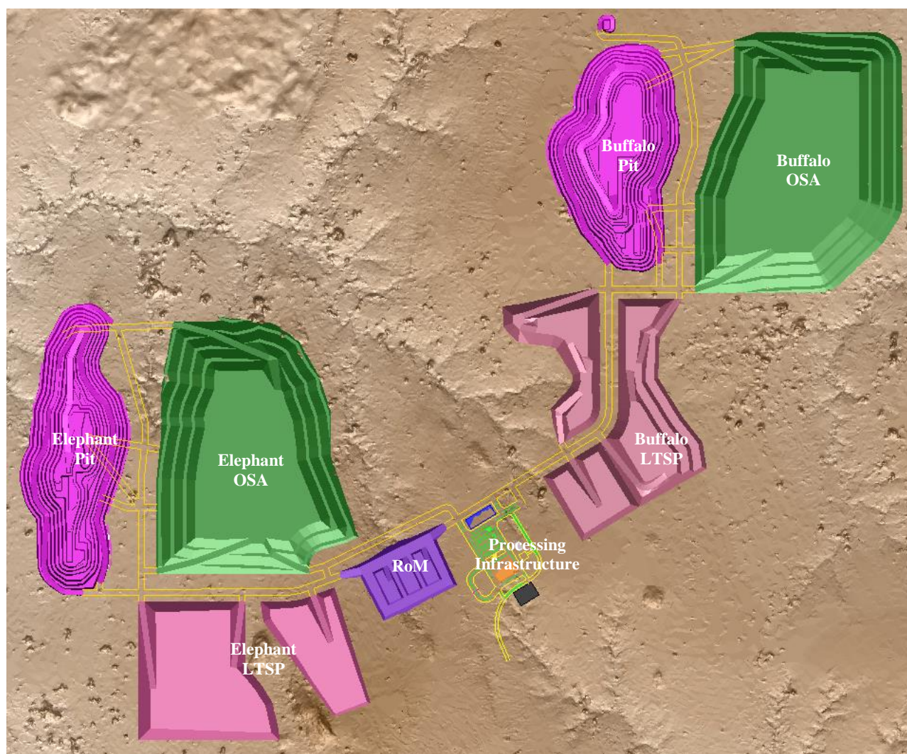
Figure 2. Montepuez Graphite Project: Mine & Processing Site Layout.
