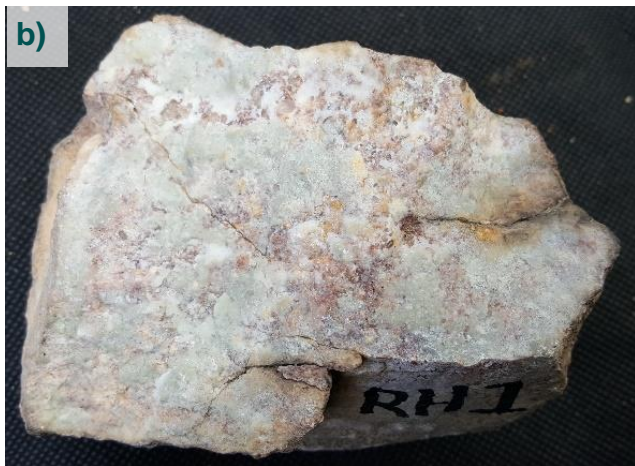
Figure 4: Such Wow prospect – Alteration features of the Shiba Zone a) Structurally-controlled pervasive bleaching in very coarse Mamadawerre sandstone b) Diaspore vein in bleached sandstone (based on portable XRF data), field of view ~ 10cm c) Pronounced clay alteration of very coarse sandstone, field of view ~ 10cm
