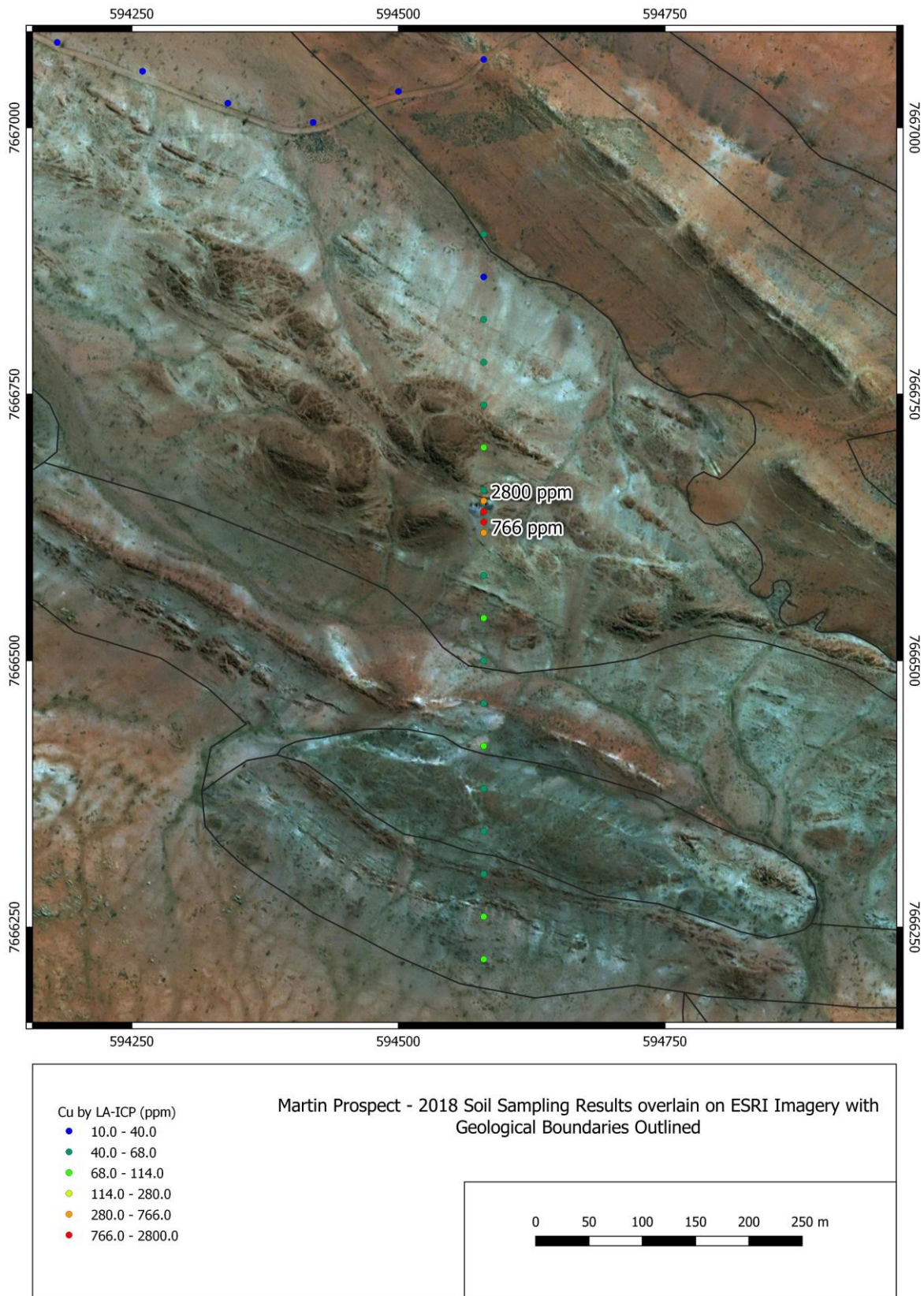
Fig 1. Distribution of copper in soil from the first-pass orientation sampling over the mafic rocks hosting the Martin copper-zinc gossan overlain on the ESRI satellite imagery.
