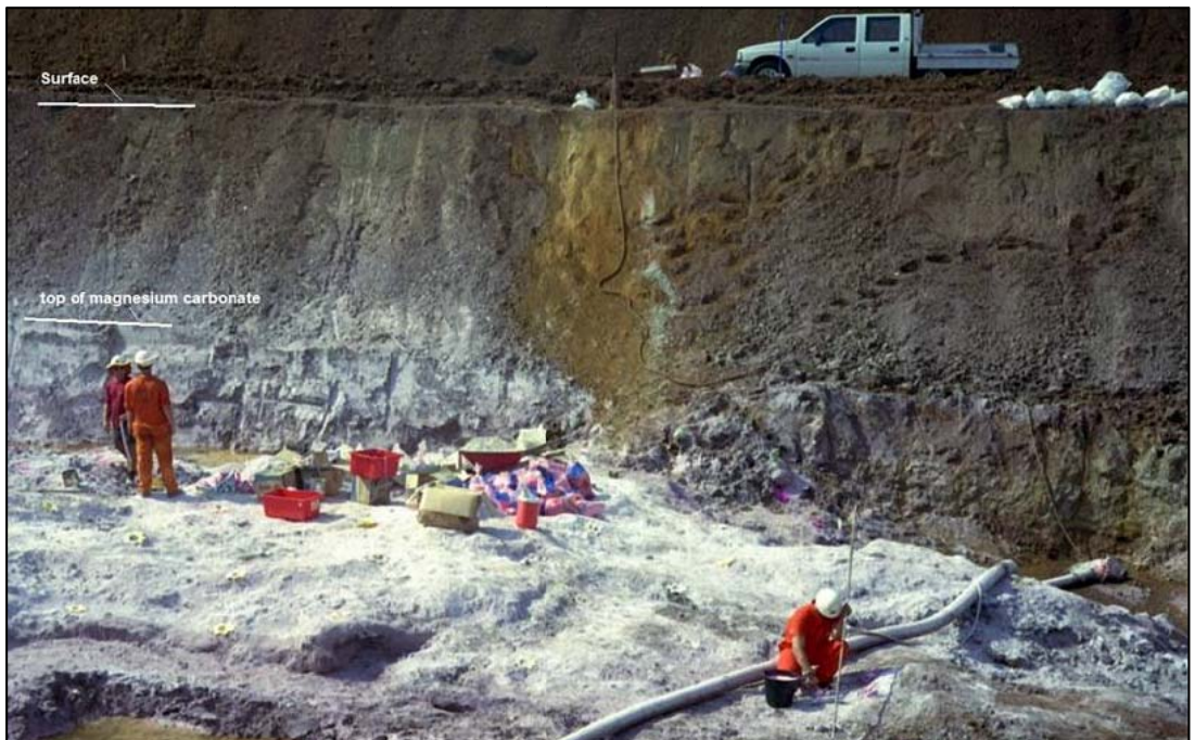
Figure 2 Test mining of magnesium carbonate at Winchester (setting of charges)
