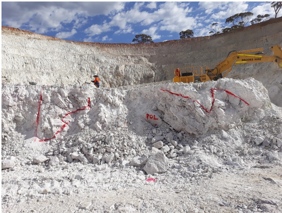
Photograph 1 - 11 th December 2018: looking north at the 297.5 flitch face, with pollucite (POL) marked out for excavation.
