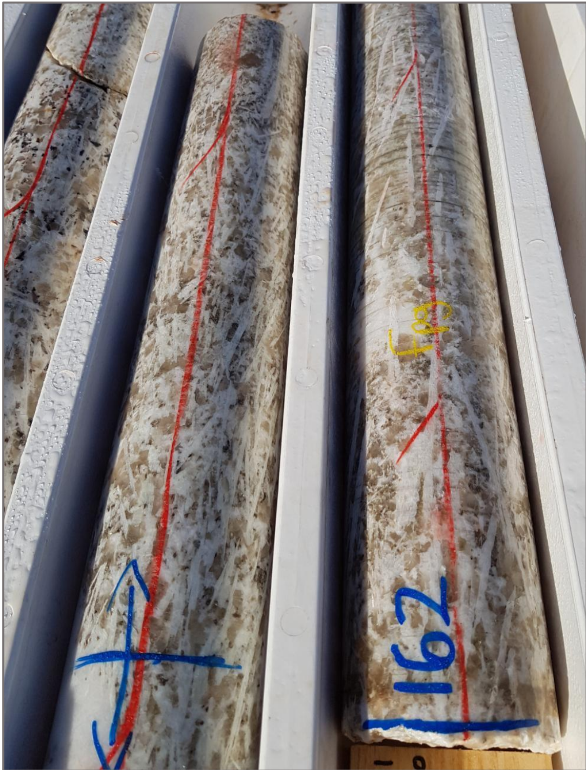
Figure 2: Kathleen Valley Project – PQ diamond drill core showing abundant white spodumene crystals (NB core diameter ~ 8.5cm)
