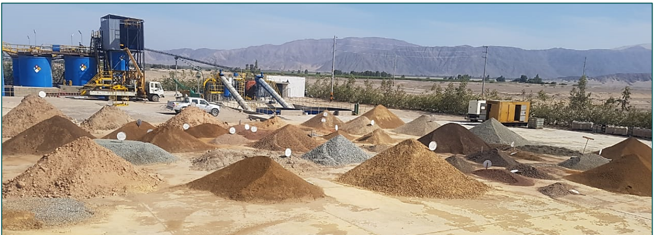
Figure 1 | Vista crushed ore stockpiles from primary crushing circuit, awaiting commissioning of secondary crushing and grinding circuit
