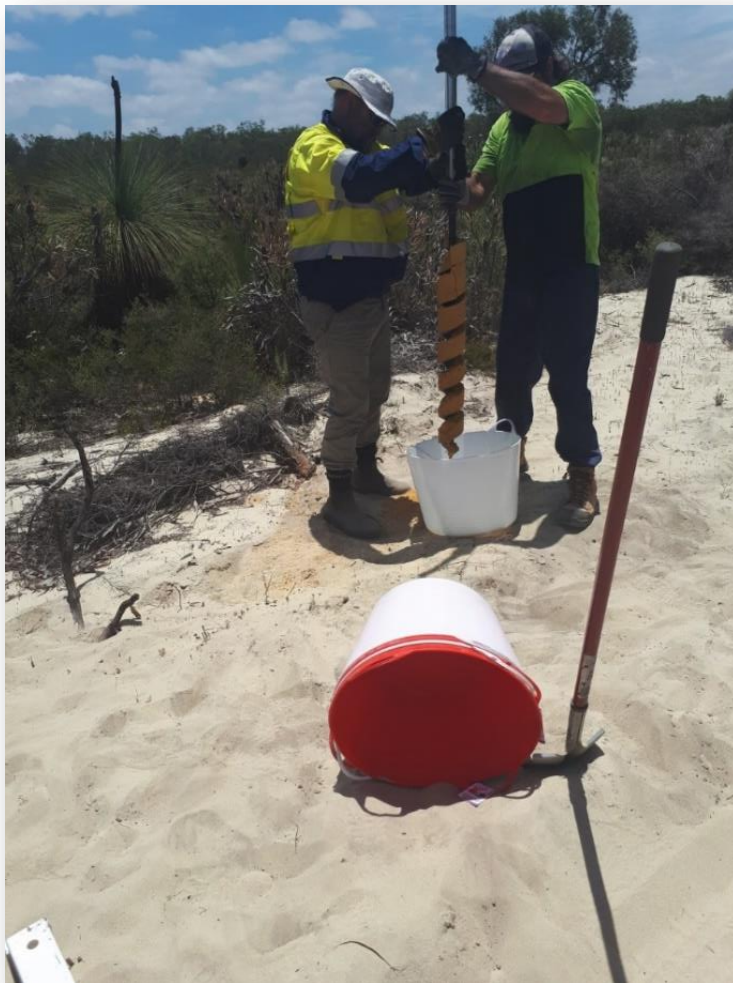
Figure 4: Hand auguring sand at Arrowsmith
