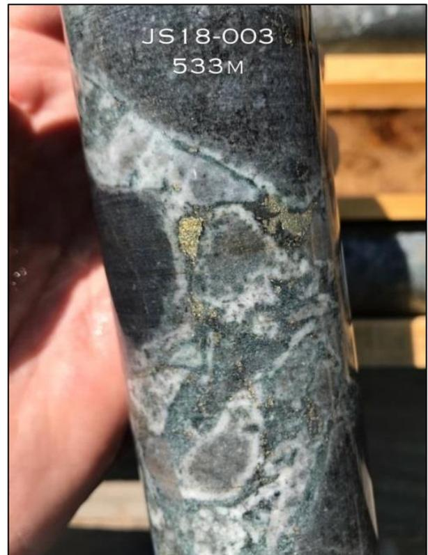
*Photo 2 B. Hydrothermal dacite breccia with albite rims on biotite-magnetite altered breccia clasts and with a sulphide-bearing chlorite matrix (hole JS18-003, 533m).*
