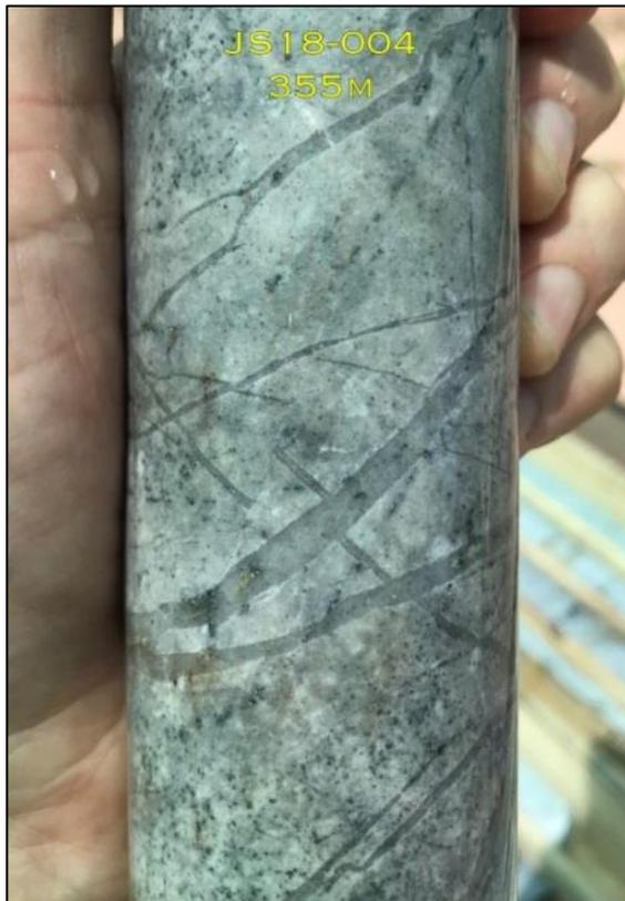
*Photo 2 A. | Silicified dacite porphyry containing molybdenite-bearing A-type quartz veins (hole JS18-004, 355m). Assays awaited.*
