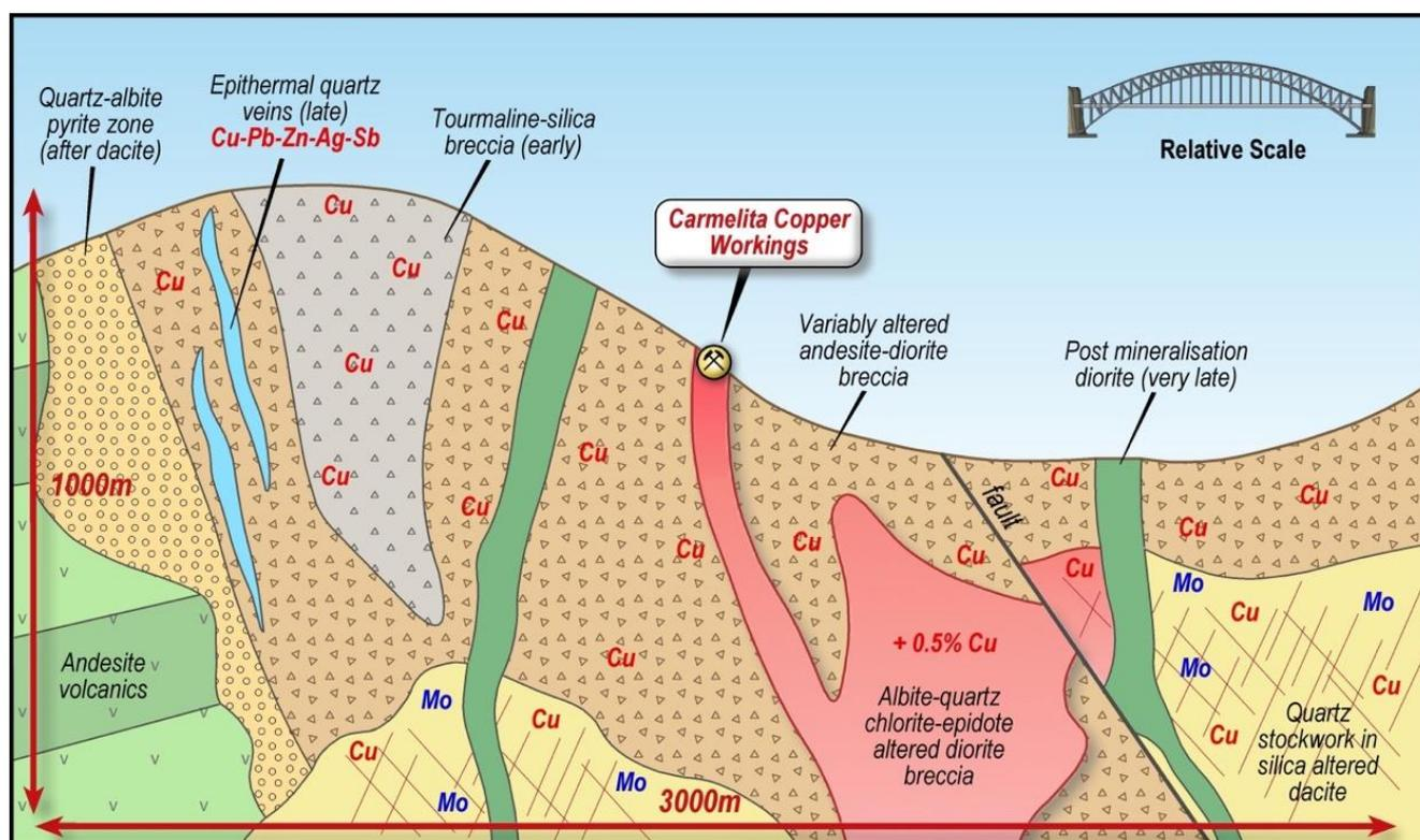
Figure 2 | Joshua Porphyry System - Interpreted schematic E-W geological model in E-W section.
