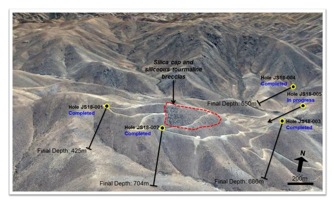
Figure 1 | Relative positions of 2018 drill holes at Joshua shown on north-looking Google image.
