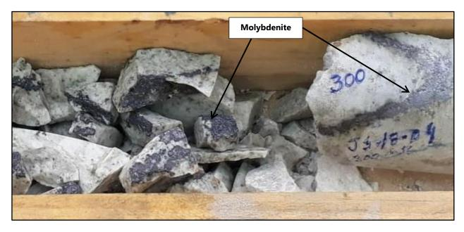
Photo 1 | Molybdenite veins in silicified dacite porphyry. Hole JS18-004, 298m to 302m. 4m at 174ppm Mo.
