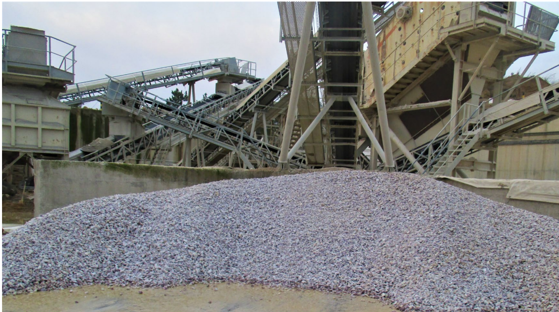
Figure 2. Crushed Alvarrões run of mine lepidolite feed.
