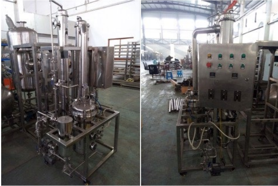
Figure 1. Pilot Plant lithium evaporator fabricated and, pending final assembly and polishing, ready for shipping.
