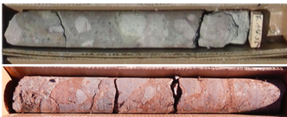
Figure 2 Core from Emu's Vidalita Prospect: Top: unoxidised polymictic breccia from hole 17DV2 (114m). Bottom: altered (oxidised) polymictic breccia from hole 17DV2 (190m). Note similarity between the core shown in the bottom image with that in Figure 1.
