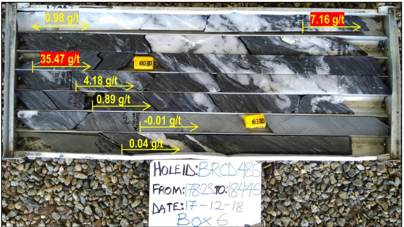
Photo 2: BRCD485 – Core run 178.23m to 184.45m
