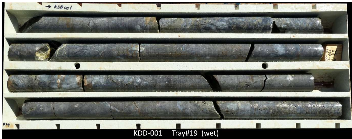
Figure 2: Hole KDD001 from approximately 61 to 68m showing extensive pervasive silicification and development of pyrite and arsenopyrite.
