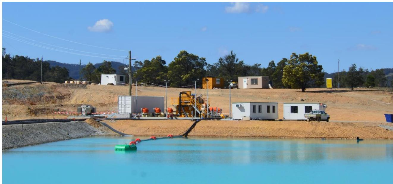
Figure 2: Hydraulic mining water reclaim, trash screen and transfer pump station
