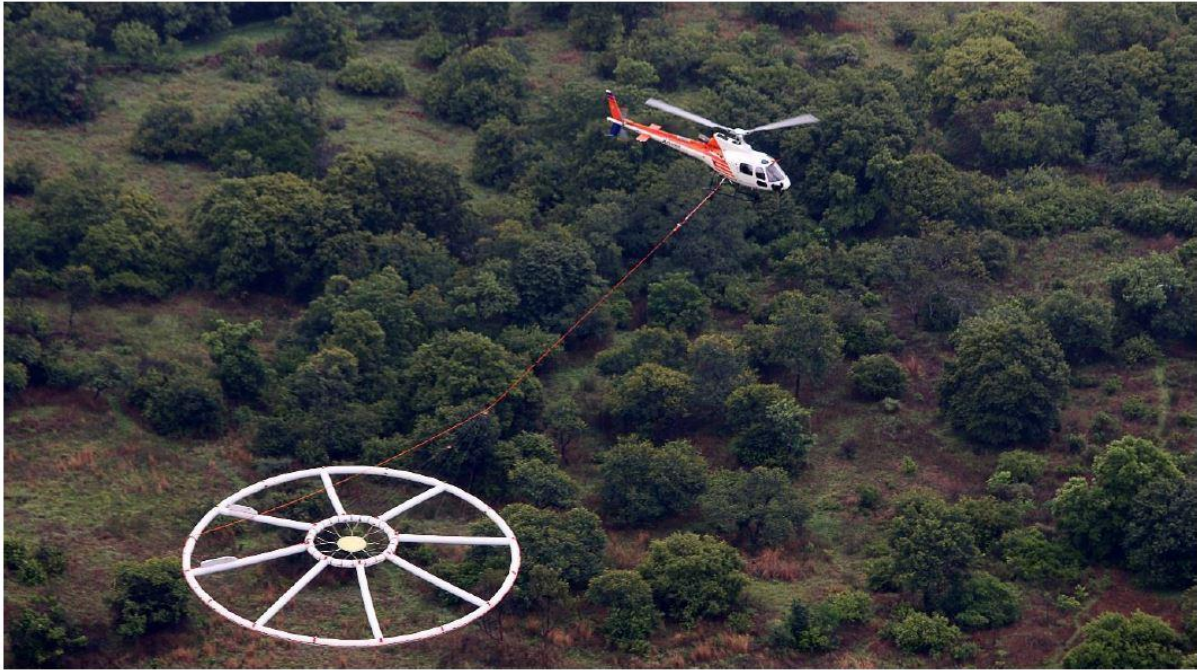
Figure 1: The Xcite airborne electromagnetic and magnetic system collects high-resolution geophysical data for targeting Bali sulphide mineralisation.
