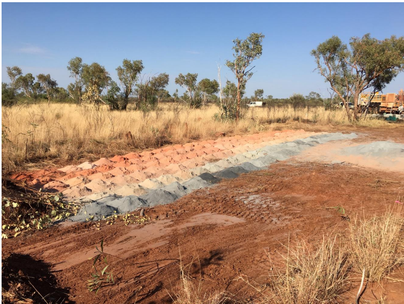
Figure 2. Quartz breccia and sulphide in SJRC0056 expressed as a dark grey colouration in RC sample piles
