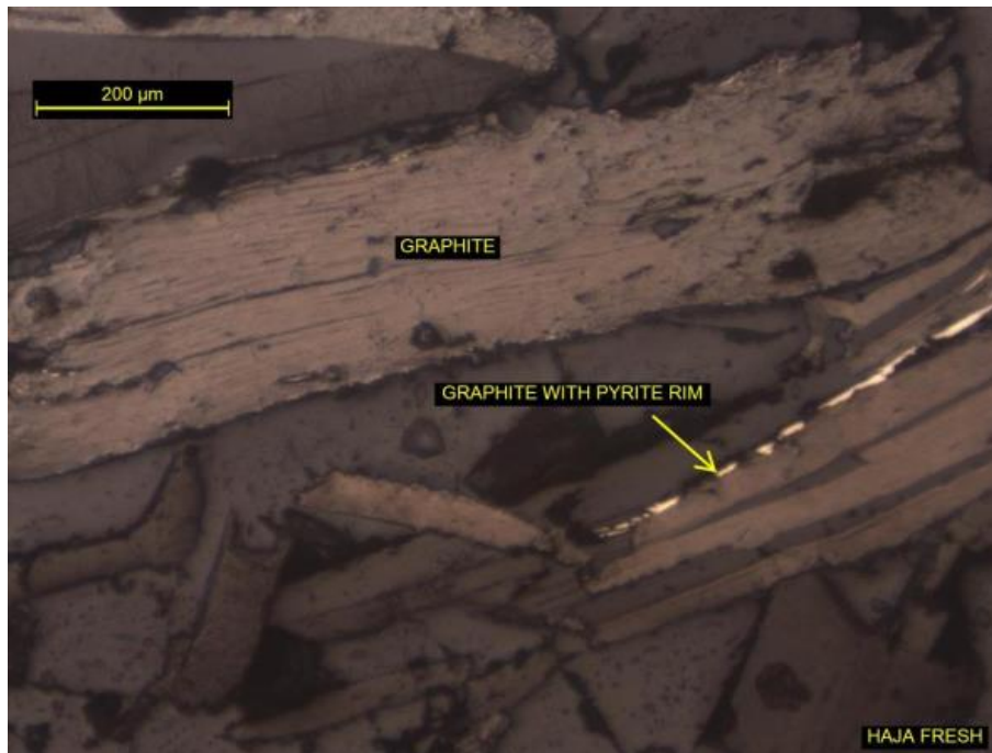
Figure 4 – Haja Polished Thin Section
