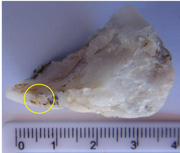
Gold in vein quartz. King of the West Mine 322356mE 6858965mN (scale marked in cm and mm)
