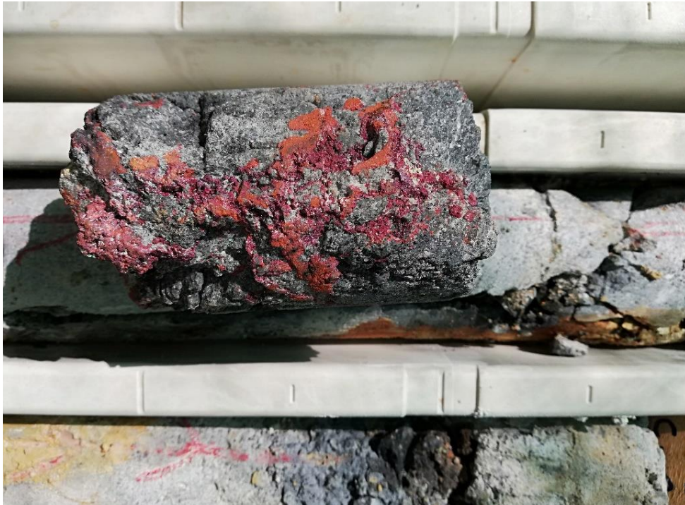
Cuprite and native copper in core, BWDD018
