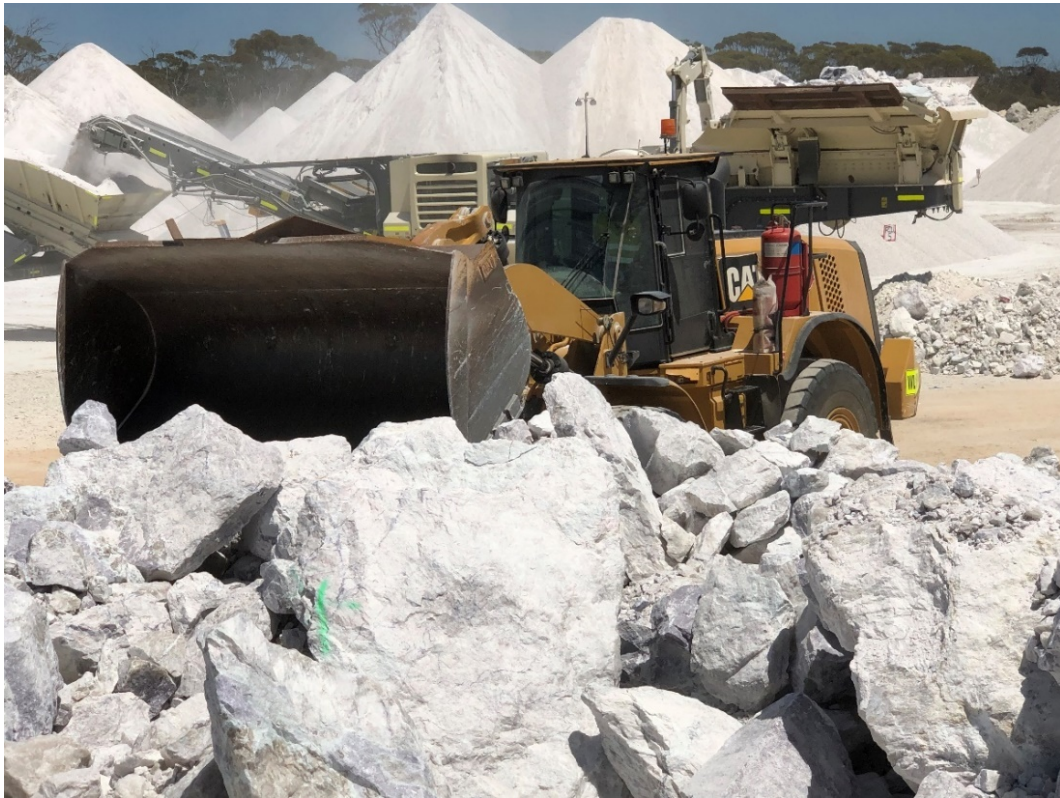
Crushing Pollucite: High grade pollucite in the foreground. In the background are the crushed ore stockpiles, each of approximately 1,200t.
