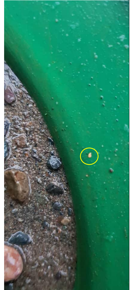
Figure 9: Gold Panned from a 5kg river gravel sample near the western edge of the lease
