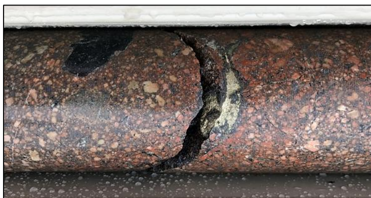
Photo 4. Chalcopyrite clot in quartz diorite porphyry with pervasive hematite (core is HQ3 – 61mm diameter).
