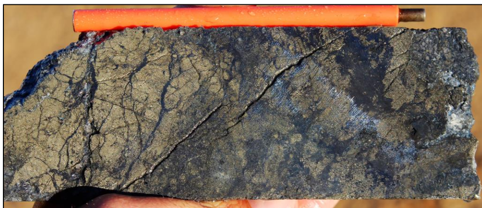
Photo 3. Basal high-sulphidation pyrite-chalcopyrite-bornite-covellite-chalcocite mineralisation from 542.5m – note the chalcocite occurs as late network veins within the more massive sulphides
