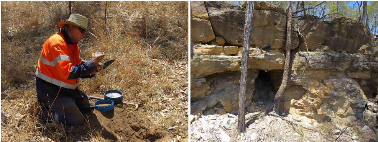
Figure 6: (left) Ultratrace sample collection. (right) Jurassic sediments overlying metamorphic basement in the Upper Camp. Ultratrace sampling is a widely used technique to locate mineralisation beneath moderate thicknesses of sedimentary cover.
