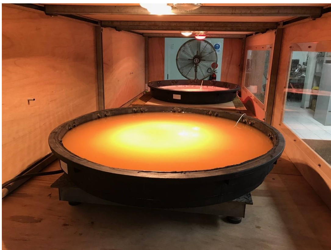
FIGURE 2 WIND TUNNEL TESTING OF LAKE WAY BRINE AT BUREAU VERITAS IN PERTH
