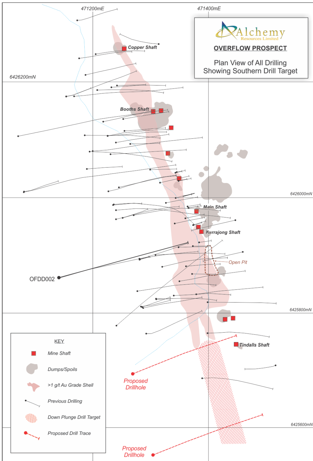
Figure 3: Overflow Prospect plan showing old workings, all existing drill collars, Au >1g/t Au grade shell (pink), and planned diamond drill holes targeting high grade gold-base metal mineralisation.
