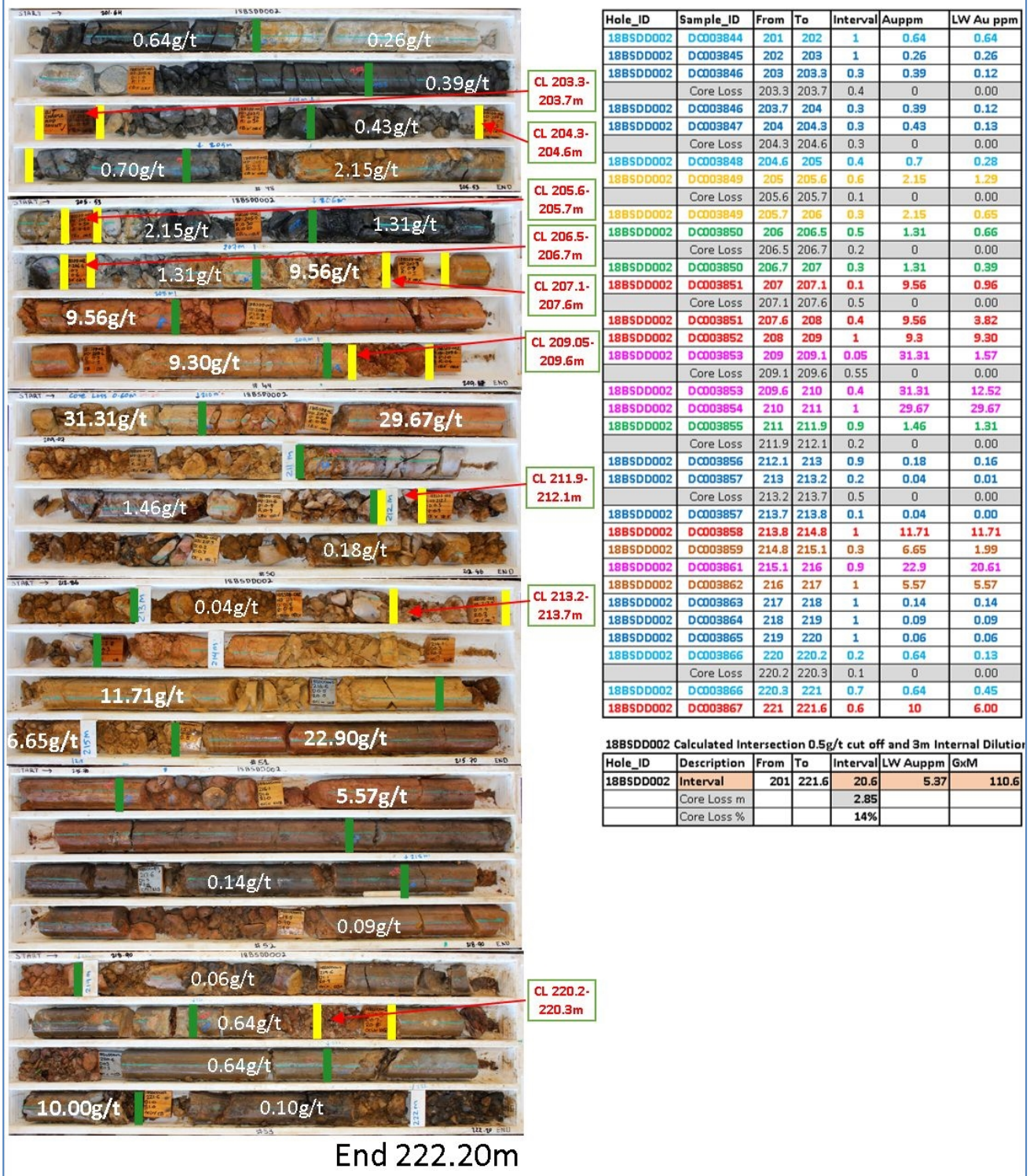
Figure 5 18BSDD002 assay labelled core photos, of mineralised intersection 201m to 221.6m. Shows strong weathering/oxidation of the host shear zone and intervals of mineralisation including core loss (CL) within intervals of VHG mineralisation. All core loss has been assigned 0g/t Au grade and a conservative length weighted intersection calculated using 0.5g/t Au cut off, 3m internal dilution
