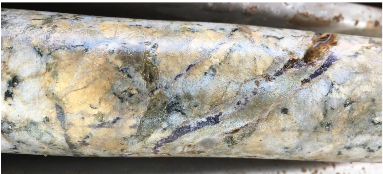
Figure 6. Fluorite+quartz-veined and altered granite drill core from Rankins Reward Prospect hole RR3 47m.
