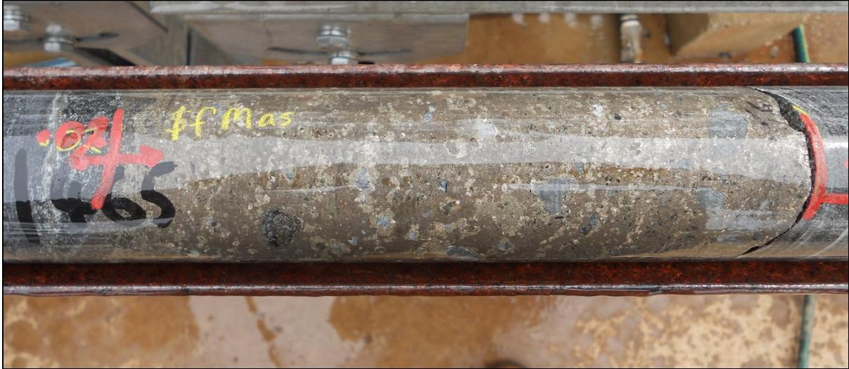
Figure 2: PLJD0006 showing mineralised tectonic breccia zone
