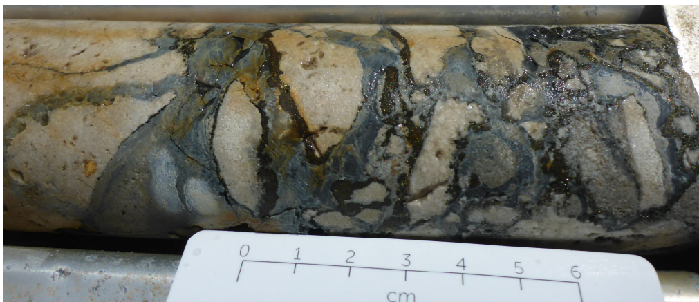
Figure 9: Close-up of WRD01 at 495.3m showing carbonate breccia hosted mineralisation with 2% Zn spot XRF with marcasite.
