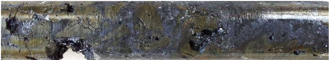
Figure 3. Massive Sulphides – Typical Galena (Grey-Blue) With Pyrite (Bronze), Diamond Core from AF005, 82.1m. Strong Lead Mineralisation is Intersected Over 9.4m Length in This Particular Hole
