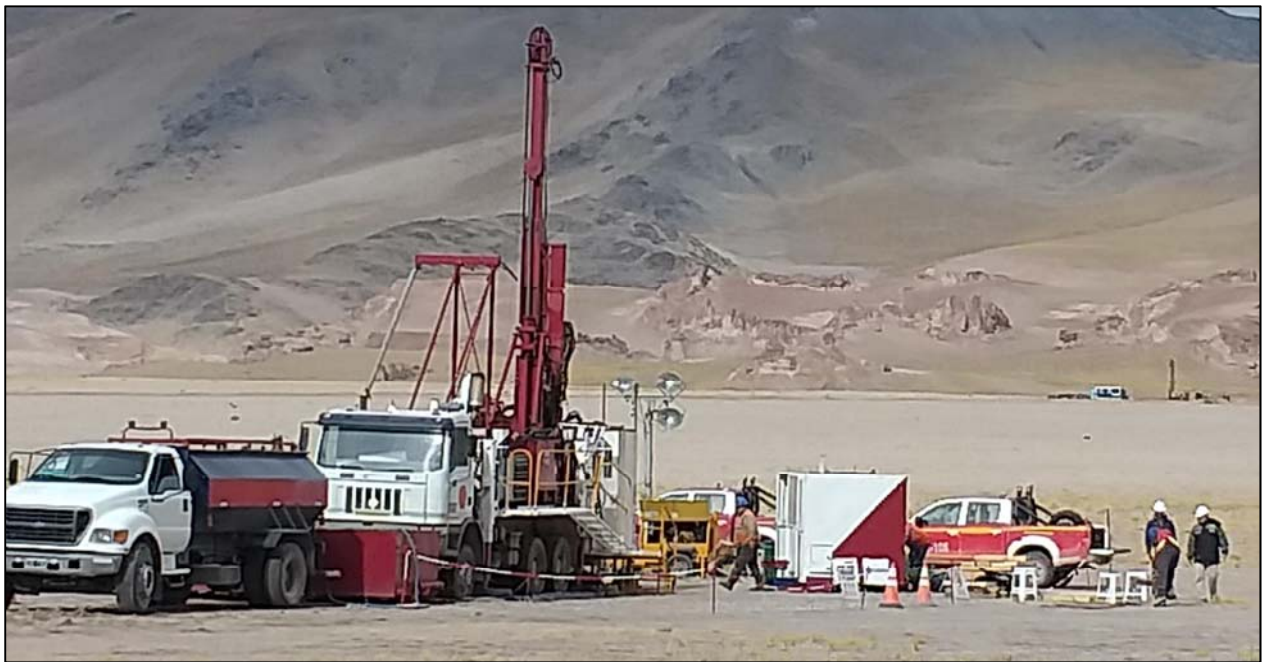
Figure 1: Diamond drill rig working at the Candelas project, Hombre Muerto, with Galaxy Resources' drill rig operating ~1km away in the background
