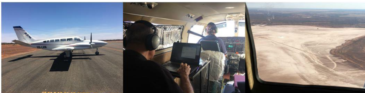
Figure 6: AAM Group flying LiDAR topographical survey over Lake Way
