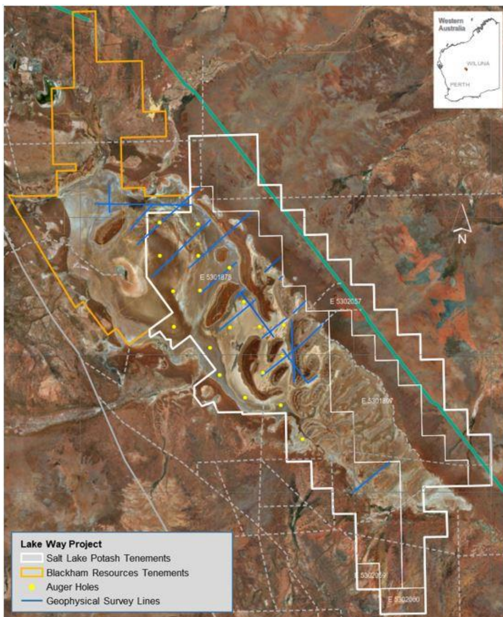
Figure 4: Location of Auger Holes and Geophysical Survey lines at Lake Way
