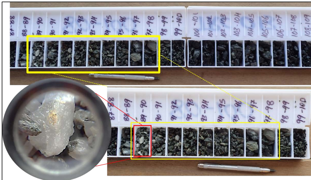
Figure 5 – Photograph of core tray from TRC013 in which record intercept of 1 m @ 251.27 g/t Au was recorded, as well as sample of visible gold from mineralised interval.
