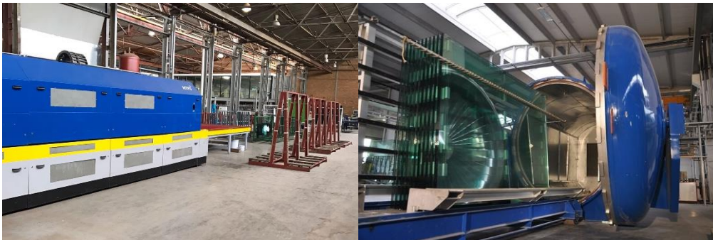
Some of Glass Partners' manufacturing facilities – toughening furnaces and glass laminating autoclave.
