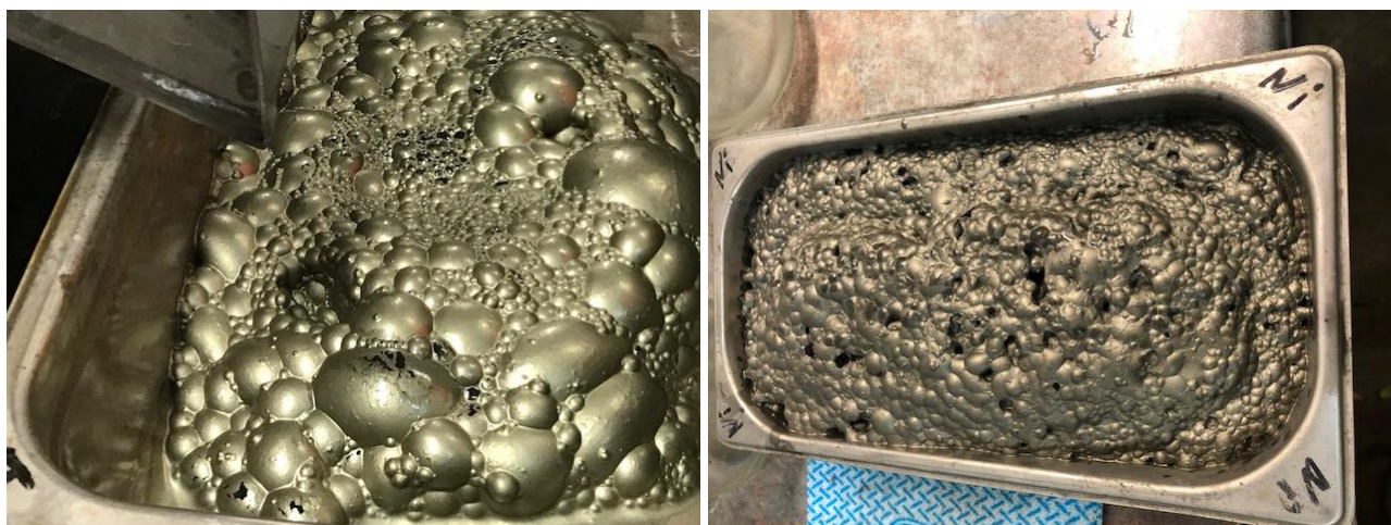
Figure 1. Final copper concentrate (left) and nickel concentrate (right) from Master Composites
