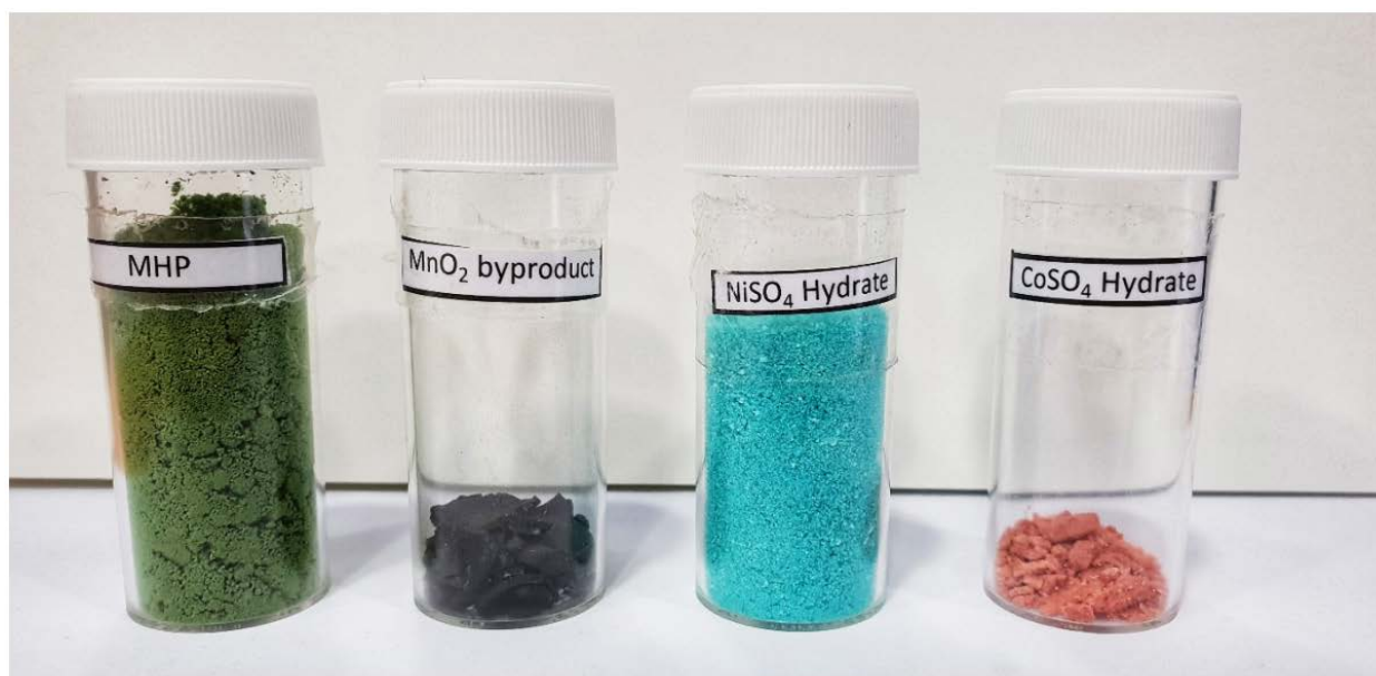
Figure 2: Nickel-Cobalt MHP from DNi Process™ (green) upgraded to produce Nickel Sulphate (blue), Cobalt Sulphate (orange-pink) and Manganese Dioxide (black)
