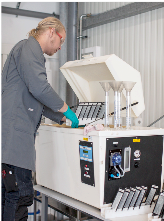
Figure 6. Talga technician performing corrosion testing of Talphene coatings at Talga Advanced Materials GmbH facility in Rudolstadt, Germany.
