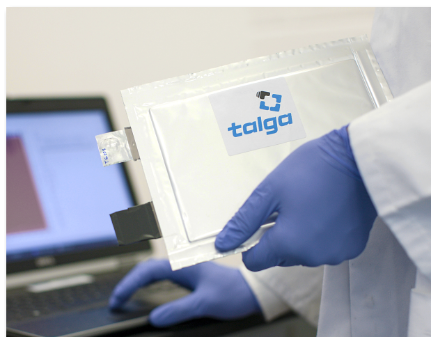
Figure 3. Lithium-ion battery pouch cell prepared with Talnode-C anode product for testing.
