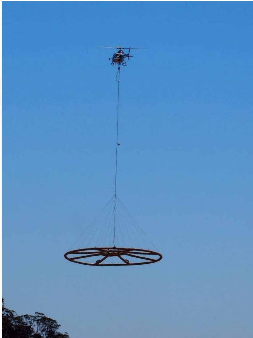
Figure 21: NRG helicopter undertaking AEM survey over E70/4688
