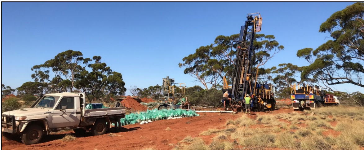
Photo 1: Reverse Circulation (RC) Drilling at Lake Roe – January 2019
