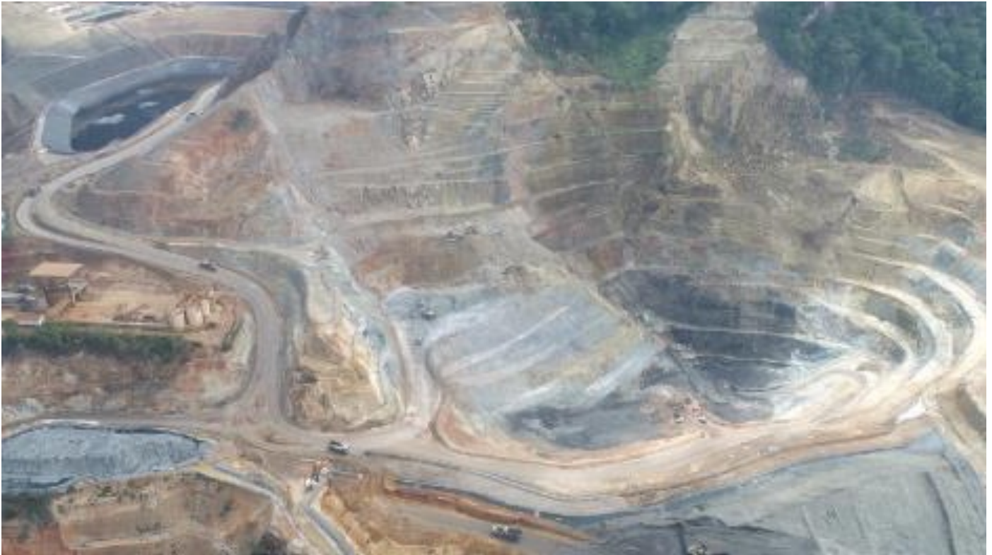
Figure 1 – Kali Kuning pit as at late December with pit wall remediation works advancing.
