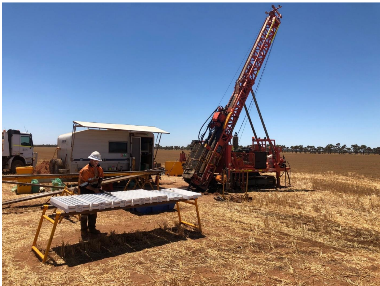
Diamond core drilling underway at Cygnus Gold's Bencubbin Project
